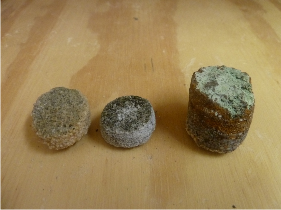
Figure 9. Core buttons (2.54 cm diameter) with case-hardened surface. Left and center samples are silica case-hardened, right sample is iron case-hardened.
