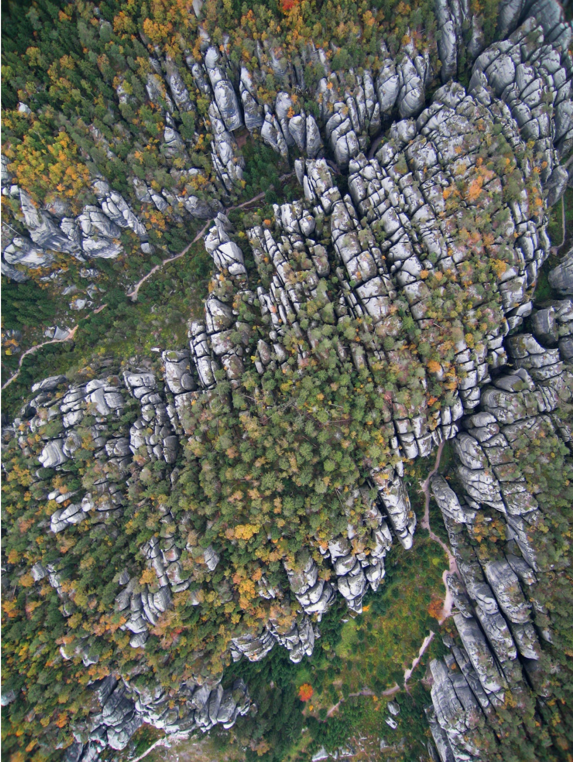
Figure 2. Non-orthographic aerial photograph of Rock Island. North is approximately at the top of the photo. Note the dominant fracture set running roughly NW-SE and conjugate fractures roughly NE-SW (see Figure 4).
